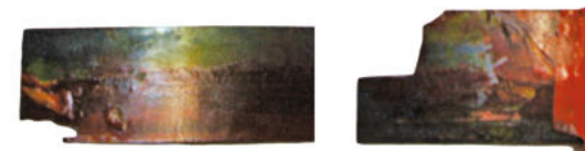
Damage to doctor blades from chipped ends
