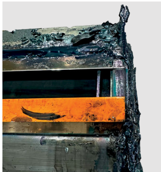
Severe end seal leaking
