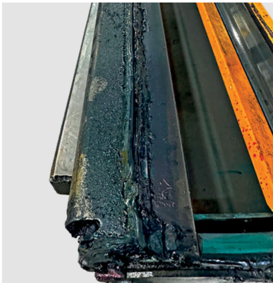
Combined leakage and buildup on the lower half of the holder
