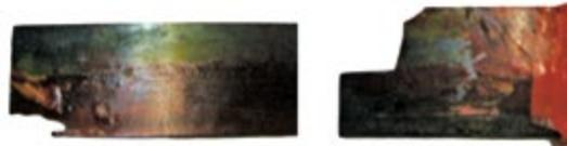
Damage to doctor blades from chipped ends
