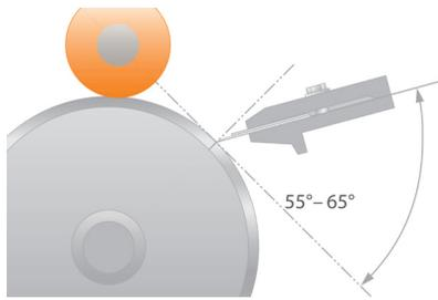
**Fine adjustments are required for optimal printing results** The gravure industry recommends a doctor blade contact angle of approximately 55 to 65 degrees.
