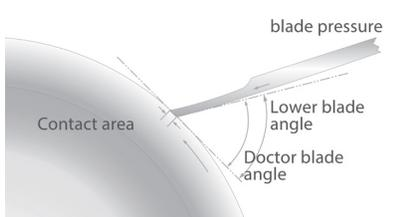
**Doctor blade pressure: Less is more** We strongly recommend using minimal doctor blade pressure. The thinner the tip, the less pressure required to achieve a clean and brilliant printing result.
