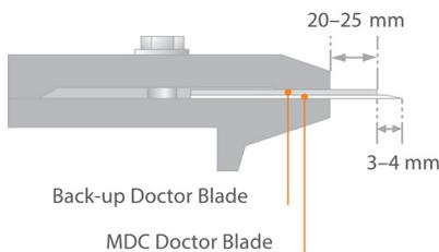
**The correct installation of the doctor blade into the doctor blade holder**
