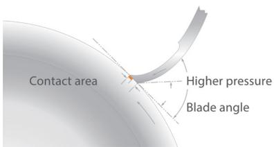
**Excessive doctor blade pressure** Too much pressure will result in excessive deflection of the doctor blade. Increased deflection creates a lower contact angle and wider contact area, which leads to hazing and tonal value changes in the printed product.
