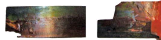
Damage to doctor blades from chipped ends
